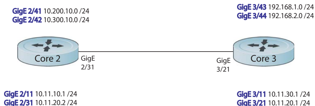
Figure 43-7. RIP Topology Example
