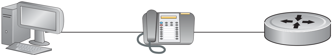
Figure 37-7. Office VOIP Deployment
